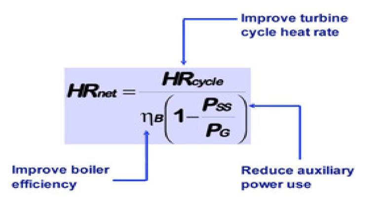
To illustrate the magnitude of this effect, a sensitivity analysis was performed for an 800-MW (gross) power plant with a turbine cycle heat rate of 8,000 Btu/kWh and boiler efficiency of 85%. The baseline auxiliary power use was 80 MW, and baseline net unit heat rate was 10,458 Btu/kWh. The results, presented in Figure 2, show that a 10% reduction in auxiliary power use will improve net unit heat rate by approximately 1.1%.
