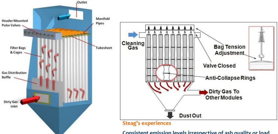
Consistent emission levels irrespective of ash quality or load Higher pressure drops(higher energy) Higher maintenance(bags replacement)
