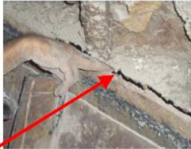
Large cracks in Bottom Hopper Seal Trough seal plates and trough connections to hoppers
