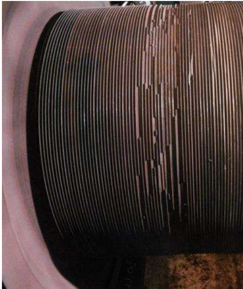
DAMAGE TO SEALS
