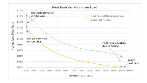
It is seen in the case of Dadri, the overall plant HR behavior was found to follow the same pattern as of original HBD calculations. The deviation from design heat rate at 100% and at 40% is found to be same (around 4%) and this deviation can be attributed to ageing of the plant.
