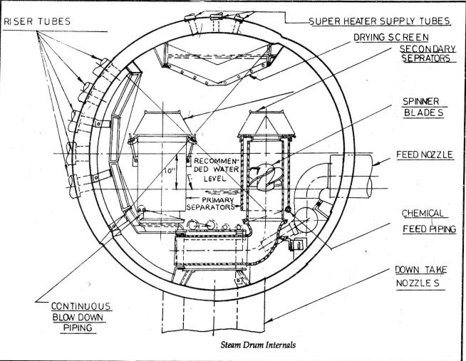
The steam drum contains steam separating equipment and internal piping for distribution of chemicals to the water, for distribution of feedwater and for blowdown of the water to reduce solids concentration.
