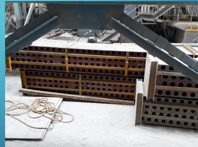
New GD screen with variable diameter holes
