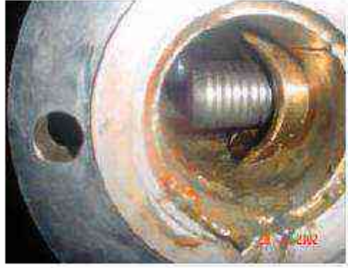
FIGURE 5 - View of Probe Installed in Tap
