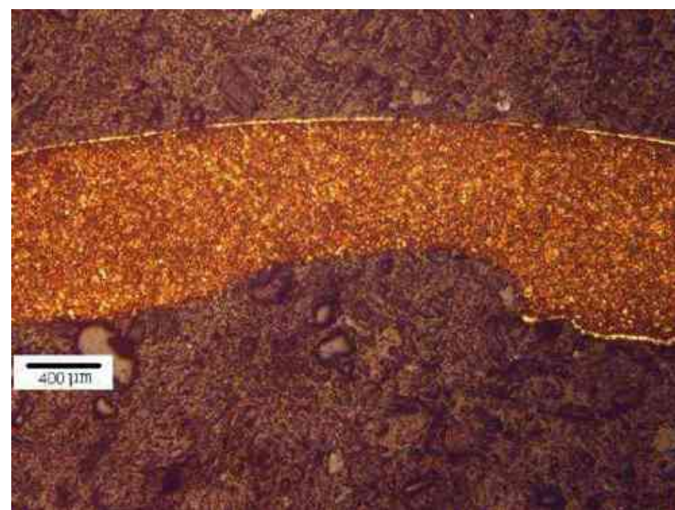
Typical microstructure of the tube surface showing severe attack
