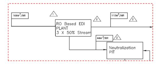
Efficiency of installed Reverse Osmosis Plant is 71 % and approx. 4 % under the standard design value
