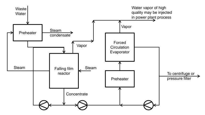
Further reduction of concentrated waste water discharge can be reached with a downstream centrifuge or pressure filter. Own consumption for 7.5 m<sup>3</sup>/h waste water is estimated to approximately 250 kWh/h, 900 kg/h steam (3bar) and 25 m<sup>3</sup>/h of cooling water.
