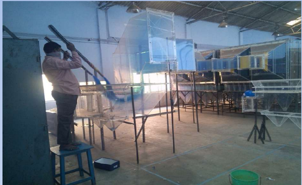
Typical physical scale model of an ESP at AQCS/BHEL, Ranipet
