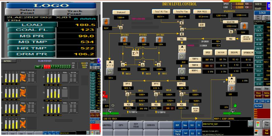
On 26<sup>th</sup> and 27<sup>th</sup> July, Load Ramp test (0.5%, 1% and 1.5%) was carried out in CMC with a specific coal consumption (SCC) of 0.61 kg/kWh. It was also in the schedule to check for the feasibility of 180 MW load.
