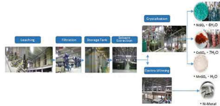
Figure 4.12: Chemical Recycling of Lithium Batteries, and the Resulting Materials
